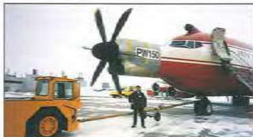
Pratt & Whitney's Boeing 720 test aircraft with PW 150 engine mounted in nose.
