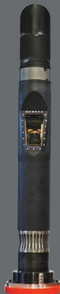
Below: Engineering Development Model (EDM) Low Profile Photonics Mast (LPPM) for evaluation on Virginia Class submarines.
