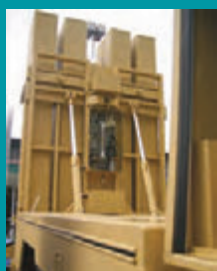
HiPPAGs are used in this vertical launch system to cool the seekers of heat-seeking missiles
