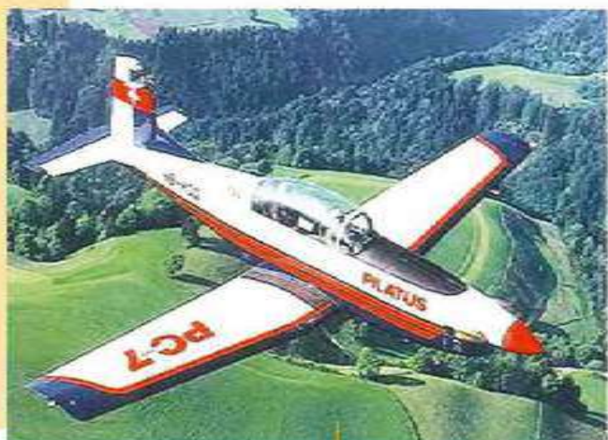
The Pilatus PC-7 aircraft – the proof of concept aircraft for the new PC-21 was built from PC-7 MkII modified to provide more jet-like handling.
